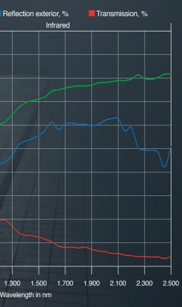
All data determined according to EN 410 and EN 673. <sup>5</sup>4 mm clear single glazing. <sup>6</sup>4/16/4 mm clear double glazing, air filled.
