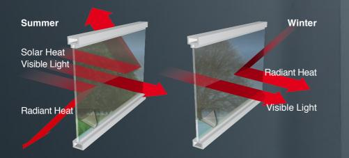
EnerLogic 35 reflects 91 % of radiant heat, EnerLogic 70 even 93 %. Therefore room temperature is comfortable all year round – it locks the heat in winter and keeps it out in summer. At the same time, EnerLogic 70 window film convinces with a fantastic light transmission.
